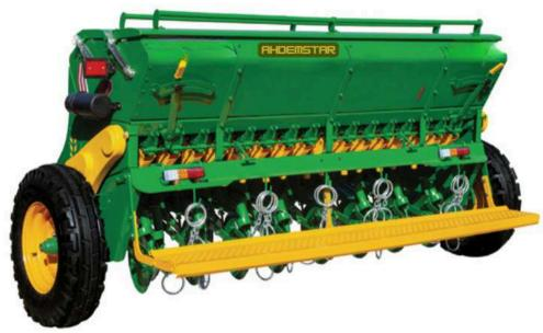
AGRICULTURAL MACHINERY TRACTOR MOUNTED SEEDER WHEAT IS SUITABLE FOR DRILLING WHEAT, BARLEY, BEANS, ALFALFA, CHICKPEA AND ETC. IT HAS FERTILIZING STORE AND CAN FERTILIZE WHILE DRILLING. IT CAN PERFORM DRILLING, FERTILIZING, COVERING AND ROLLING AT THE SAME TIME. SO IT IS A COMBINE MACHINE WHICH CAN BE LEFT AT EQUAL ROWS AND DEMANDED DEPTH AND QUANTITY TO SEEDS AND FERTILIZER.
